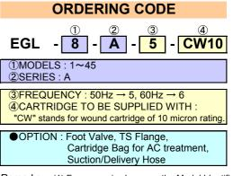
Remarks : (1) Frequency is shown on the Model Identification Plate attched on the pump.
